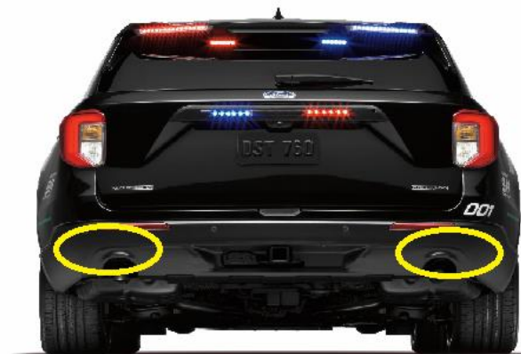
Above picture is approximate mounting location of Federal Signal 416300 Series Steady Burn lights.
