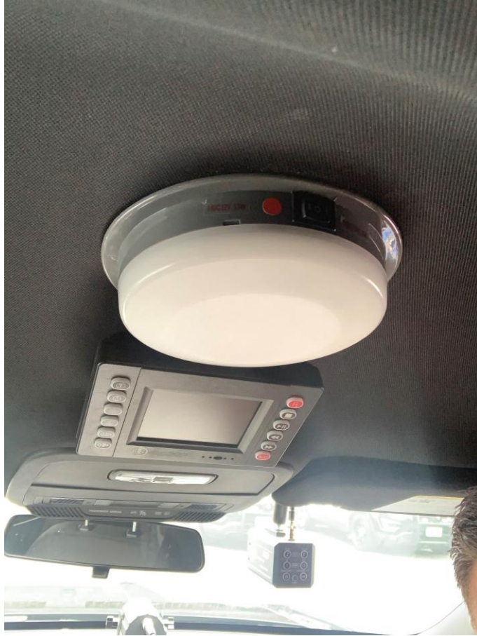
Above picture is for illustration purposes to display style of red/white switchable dome light to be mounted in front driver area and rear cargo area.
