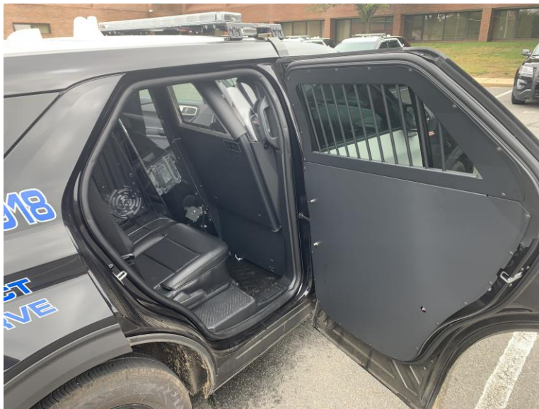
Above picture is for illustration purposes to show Vertical Window Barriers, flat panel, partition and cage style.
